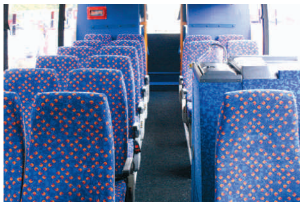
Seating for 24 passengers is retained in both the front and rear sections. Customers are assigned a seat and a bunk. Note the toilet compartment with its hot drinks dispenser and fridge.
