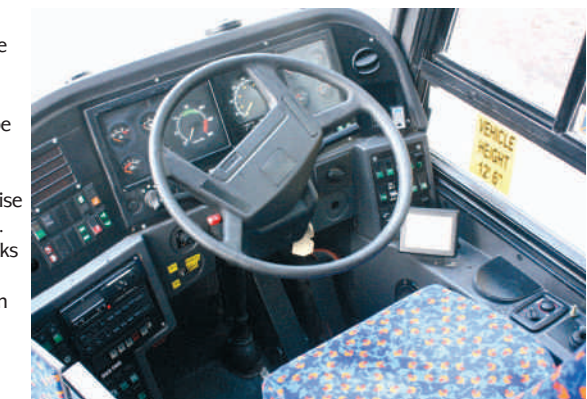
Cab of the vehicle showing the CCTV screen.
