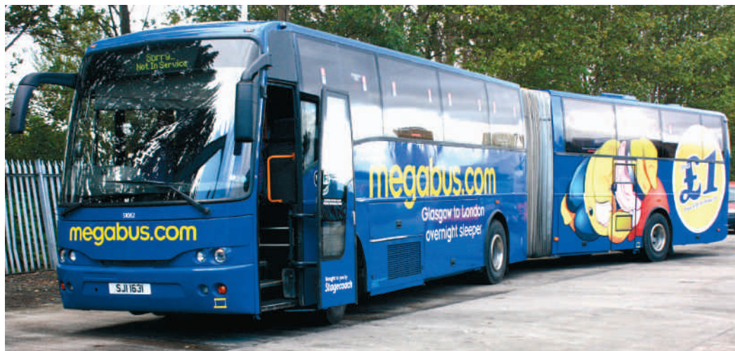
One of the Jonckheere bodied Volvo B10m articulated coaches which have been converted into sleeper coaches.
